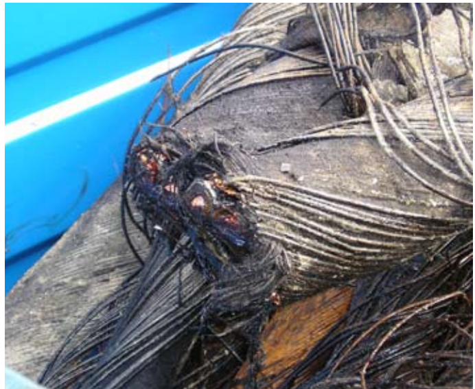
Remote control cutting underwater in the Gulf of Mexico at a depth of 762 m.
